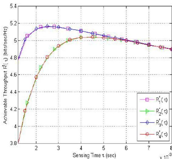
**Figure 4.2: Performance toward sensing time for different necessary interface conditions and channel noise.**
