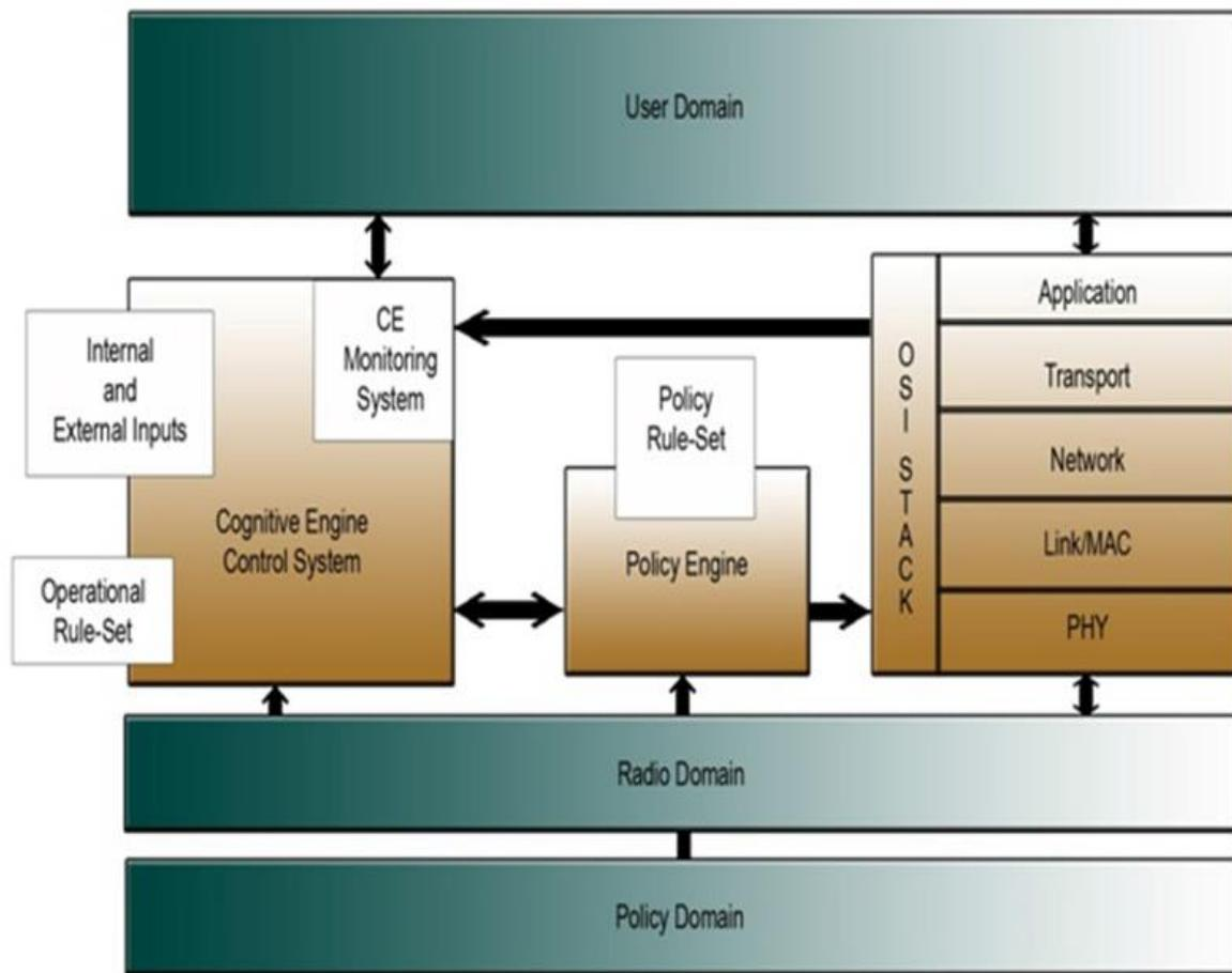
Figure 1: Cognitive Radio Concept Architecture. (Devillers, B., et al2018)
