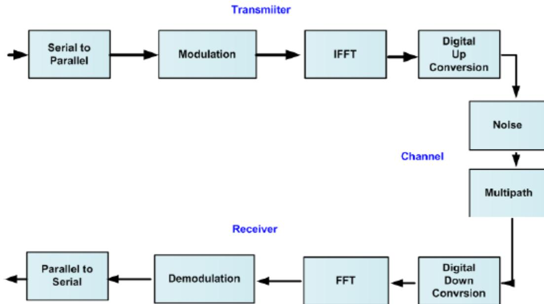
**Figure 2: Orthogonal Frequency Division Multiplexing (OFDM) Architecture. (Hubert, A. et al., 2015)**
