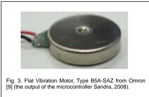
Fig. 3. Flat Vibration Motor, Type B5A-SAZ from Omron [9] (the output of the microcontroller Sandra, 2008).
