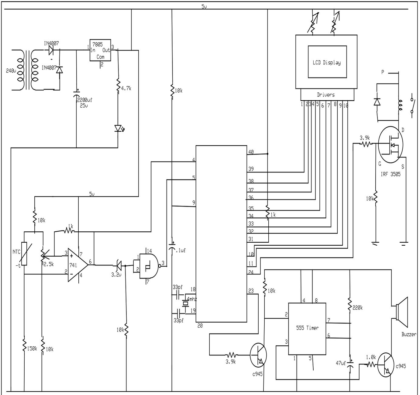
Figure 2 Complete Circuit / Schematic Diagram of the Control and Security System
